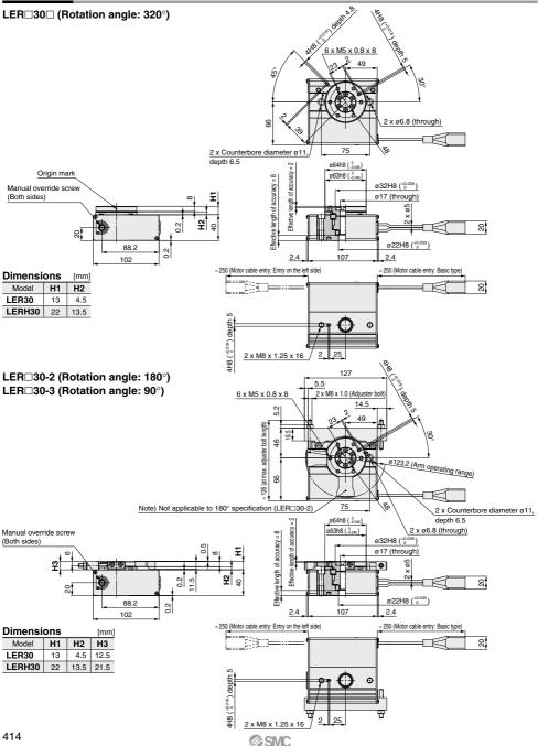
Electric Rotary Table LER Series Step Motor (Servo/24 VDC)
