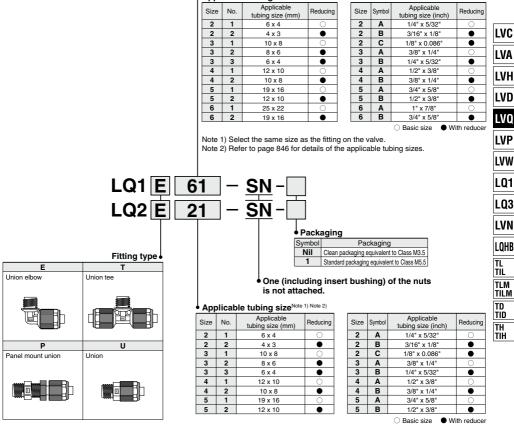
Note 1) Select the same size as the fitting on the valve. Note 2) Refer to page 846 for details of the applicable tubing sizes.
