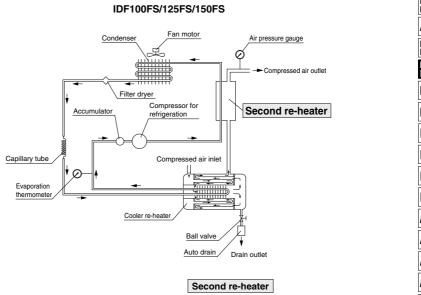
Compressed air from which drainage has been exhausted exchanges heat with refrigerant which has been compressed by the refrigerator, to give the following effects:
