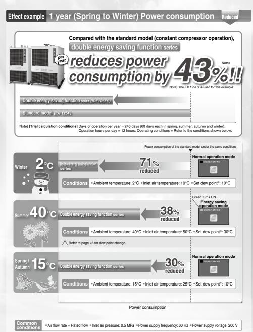
\* Dew point can be set for the double energy saving function series only. The dew point setting function is not equipped with the standard model.
