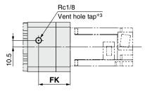
\*3 When using the dust-tight/water-jet-proof (IP65 equivalent), correctly mount the fitting and tubing to the vent hole tap, and then place the end of the tubing in an area not exposed to dust or water. The fitting and tubing should be provided separately by user. Select [Applicable tubing O.D.: ø4 or more, Connection thread: Rc1/8].
