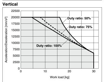
These graphs are examples of when the standard motor is mounted. Determine the duty ratio after taking into account the load factor of the motor or driver to be used.
