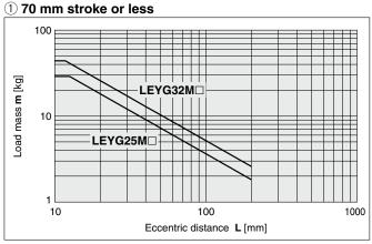
\* The limit of vertical load mass varies depending on "lead" and "speed." Check the "Speed–Vertical Work Load Graph" on page 103.
