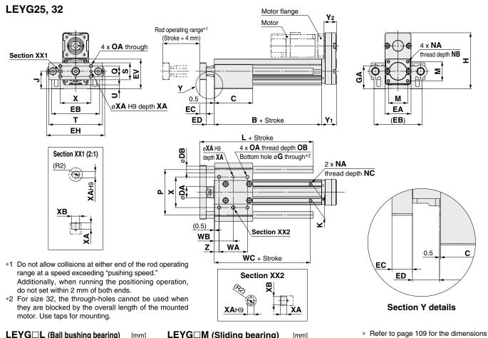
LEYG L (Ball bushing bearing) [mm] Stroke range [mm] DB L Up to 110 91 115 to 190 115 10 195 to 300 133 Up to 110 97.5 115 to 190 116.5 13
