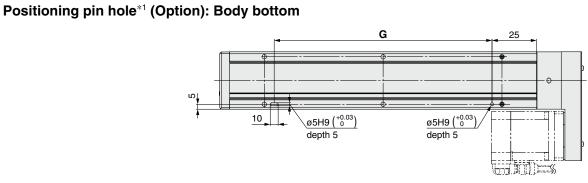
\*1 When using the body bottom positioning pin holes, do not simultaneously use the housing B bottom pin hole.
