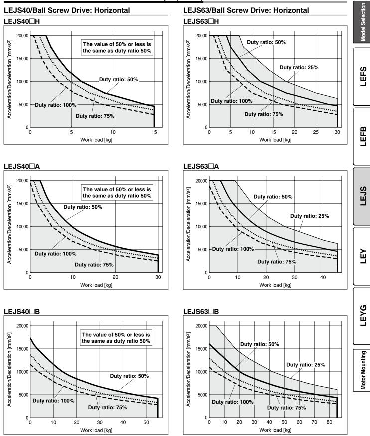
These graphs are examples of when the standard motor is mounted. Determine the duty ratio after taking into account the load factor of the motor or driver to be used.
