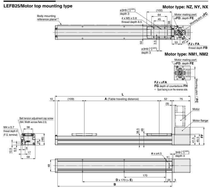
\*1 When mounting the actuator using the body mounting reference plane, set the height of the opposite surface or pin to be 3 mm or more. (Recommended height 5 mm)
