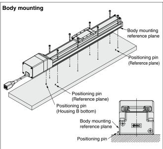
The traveling parallelism is the reference plane for the body mounting reference plane. If the traveling parallelism for a table is required, set the reference plane against parallel pins, etc.
