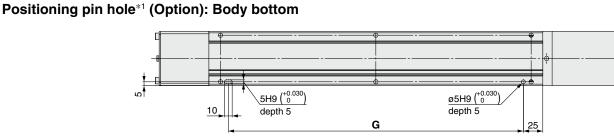
\*1 When using the body bottom positioning pin holes, do not simultaneously use the housing B bottom pin hole.
