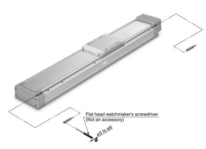
\* When tightening the auto switch mounting screw (included with auto switch), use a watchmaker's screwdriver with a handle diameter of about 5 to 6 mm. Model Selection
