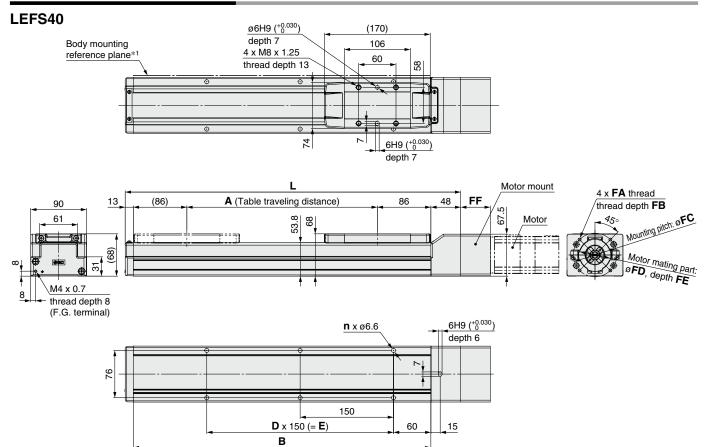
\*1 When mounting the actuator using the body mounting reference plane, set the height of the opposite surface or pin to be 3 mm or more. (Recommended height 5 mm)
