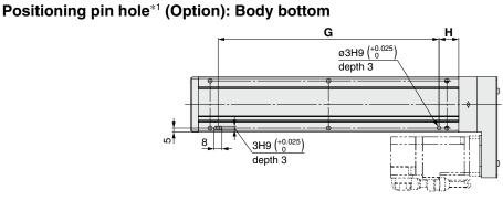
\*1 When using the body bottom positioning pin holes, do not simultaneously use the housing B bottom pin hole.
