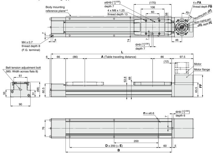
\*1 When mounting the actuator using the body mounting reference plane, set the height of the opposite surface or pin to be 3 mm or more. (Recommended height 5 mm)
