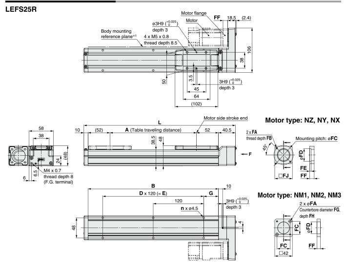
\*1 When mounting the actuator using the body mounting reference plane, set the height of the opposite surface or pin to be 3 mm or more. (Recommended height 5 mm)
