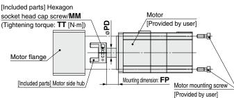
\* Note for mounting a motor to the NM2 motor type Motor mounting screws for the LEFS25 are fixed starting from the motor flange side. (Opposite of the drawing)
