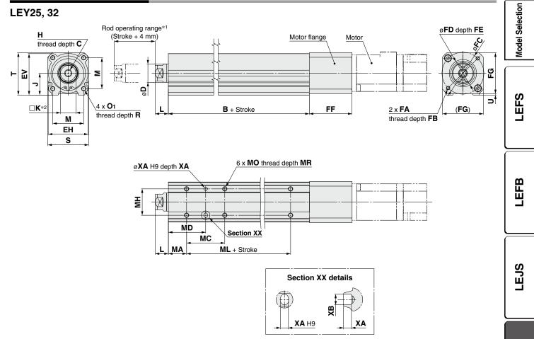
\*1 Do not allow collisions at either end of the rod operating range at a speed exceeding "pushing speed." Additionally, when running the positioning operation, do not set within 2 mm of both ends.
