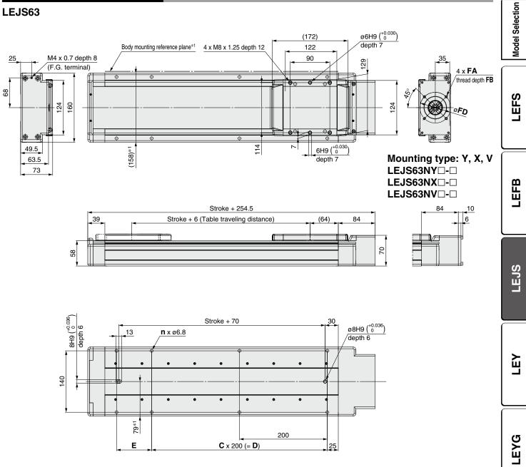
$\ast 1$  When mounting the actuator using the body mounting reference plane, use a pin. Set the height of the pin to be 5 mm or more because of round chamfering. (Recommended height 6 mm)
