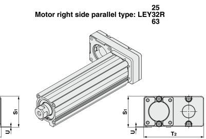
\* When the motor is mounted on the left or right side in parallel, the groove for auto switch on the side to which the motor is mounted is hidden.
