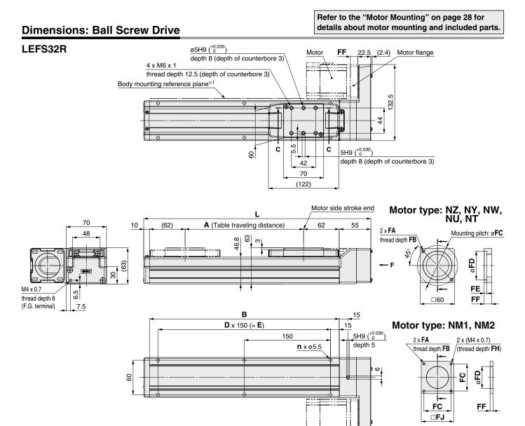
\*1 When mounting the actuator using the body mounting reference plane, set the height of the opposite surface or pin to be 3 mm or more. (Recommended height 5 mm)
