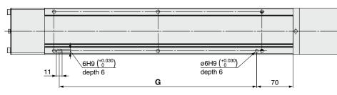
\*1 When using the body bottom positioning pin holes, do not simultaneously use the housing B bottom pin hole.
