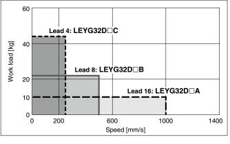
Speed-Horizontal Work Load Graph \* These graphs show the work load when the external guide is used together. When using the LEYG alone, refer to pages 101 and 102.
