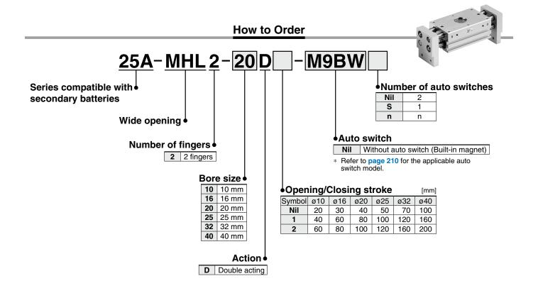
\* The 25A- series specifications and dimensions are the same as those of the standard model. (Weight is not the same.)
