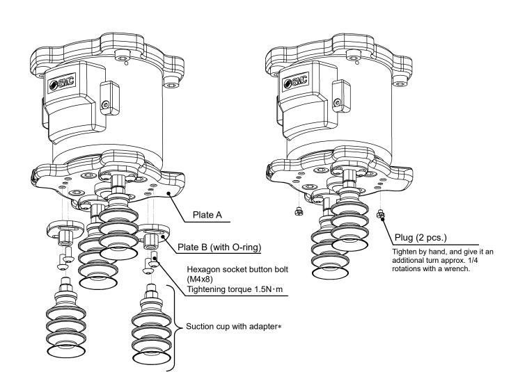
(1) Disassemble the suction cups with adapter
