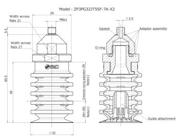
Note1) "D" and (st) indicate the reference value during adsorption at vacuum pressure: -85[kPa].
