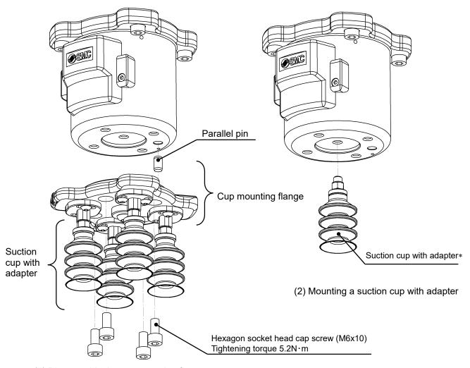
(1) Disassemble the cup mounting flange
