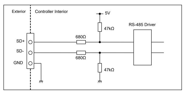
Note 1) There is no terminal resistor built into the controller communication circuit.
