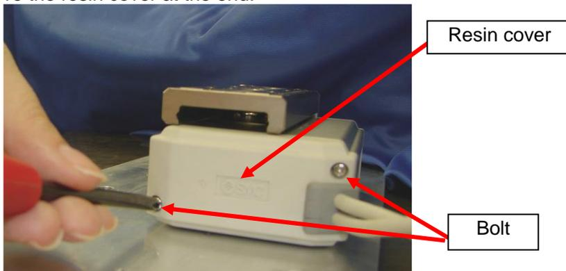
2. Displace the cover holding the cable. (If the cable is pulled forcefully, it will be disconnected)
