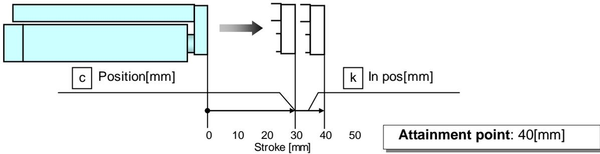
Condition 2) In case the pushing operation is **Step no.1** to **Step no.2**.
