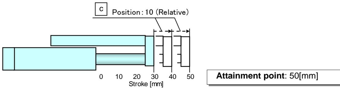
Condition 2) 30mm position → **Step no.1** → **Step no.1** (Move M: Relative)
