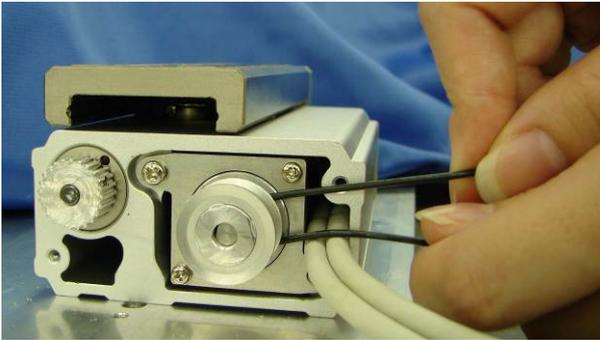
6. Set a new belt. Mount the motor pulley with belt tension force below.
