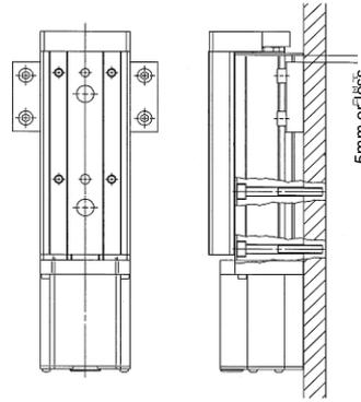
20. **The product should be mounted as shown below in the figures marked with the O.** Unstable mounting of the product may cause operation failure, generation of abnormal noise or increase in the deflection etc.
