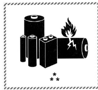
* Place for UN number (s) ** Place for telephone number for additional information Fig. app. 2 Example of label with battery illustration (Available from January 1, 2017)
