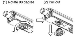
Removal procedure of emitter cartridge
