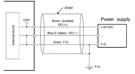
When the product is used in DC mode, make sure to ground the F.G. cable (green) and DC(-) cable (blue) of the input power supply with a resistance of 100 ohms or less. Without grounding the DC(-) cable, this products and/or power supply may be damaged.
