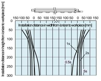
4) With Energy saving high-efficiency cartridge, Supply pressure: 0.3 MPa For IZT40-□V, IZT41-□V
