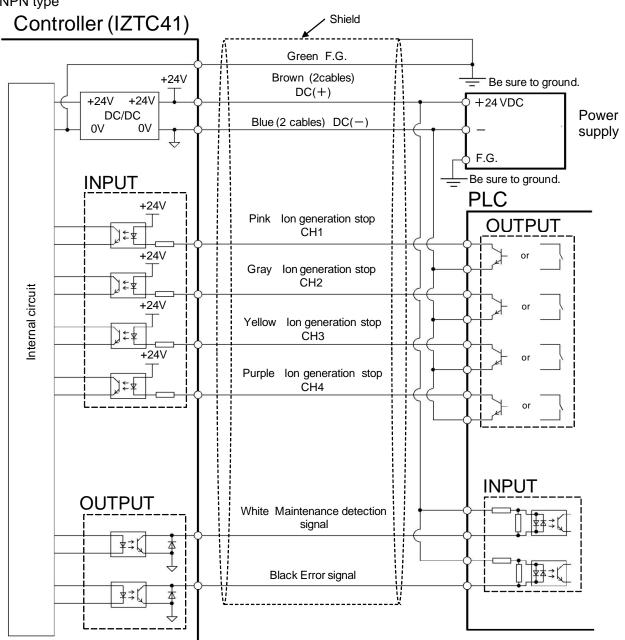
When an ionizer (IZT41) is used in DC mode, make sure to ground the F.G. cable (green) and DC(-) cable (blue) of the input power supply with a resistance of 100 ohms or less. Without grounding the DC(-) cable, this products and/or power supply may be damaged.
