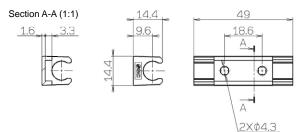
(Recommended screw: Cross recessed pan head screw M4 x 5)
