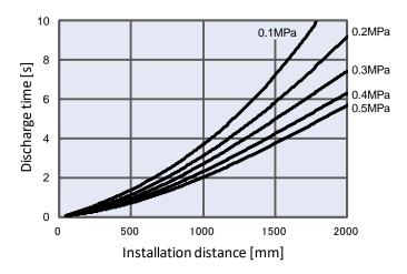
2) With High speed static neutralization cartridge With air purge, For IZT42-112D
