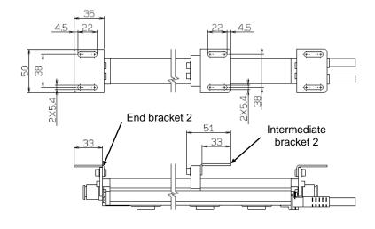
With High speed/ Energy saving static neutralization cartridge
