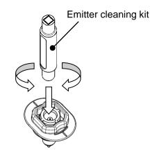
d. When the emitter cartridges are removed for cleaning, remount them to the bar according to the "Mounting procedure of emitter cartridge" shown below. Make sure that the cartridges are securely mounted. If not, the cartridges may become dislodged when compressed air is supplied to the ionizer.
