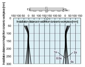
3) With Energy saving static neutralization cartridge, Supply pressure: 0.3 MPa For IZT42-□L
