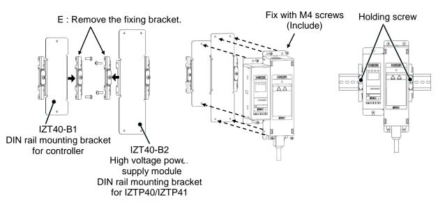
I . When the controller and high voltage power supply module are connected by separate cable · Mount the spacers to the high voltage power supply module connector. Refer to 3-1-6. Connect the controller and high voltage power supply module.
