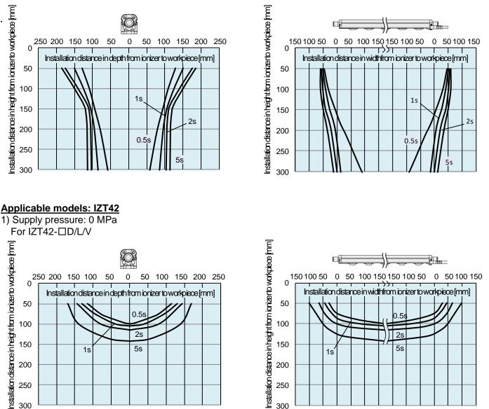
With High speed static neutralization cartridge, Supply pressure: 0.3 MPa For IZT42-□D
