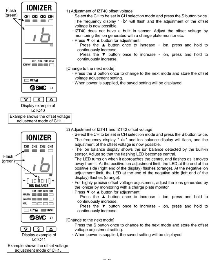
The selected bar (high voltage power supply module) moves on to the ion generation stop mode by pressing
