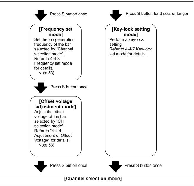
Note 53) In Channel selection mode, frequency set mode, or offset voltage adjustment mode, the selected bar (high voltage power supply module) moves on to the ion generation stop mode by pressing  $\vee$  and  $\blacktriangle$  button simultaneously for 2 s or longer and stops the ion generation. (Operation is not possible while the key lock is ON). To release, press the S button once or turn the power off and on again. Refer to [ 4-4-8. ion generation stop mode] for further details
