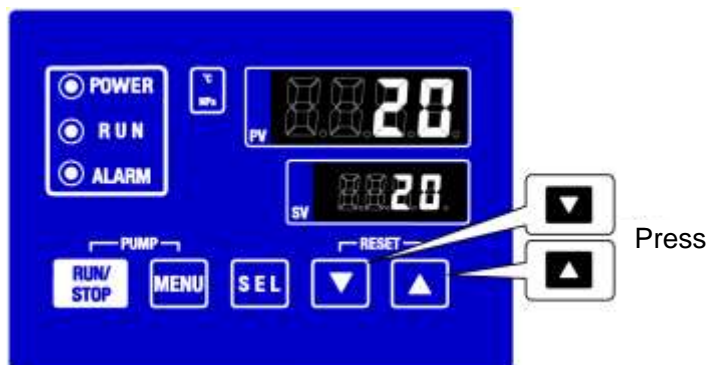
Fig. 4.2-2 Setting of circulating fluid temperature
