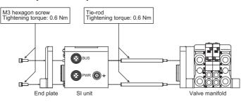
Exchange of SI unit •Remove screws from End Plate and release connection of each unit. •Replace old SI unit with new one. (Tie-rod does not need to be removed.) •Connect Input Block and End Plate and tighten removed screws by specified
